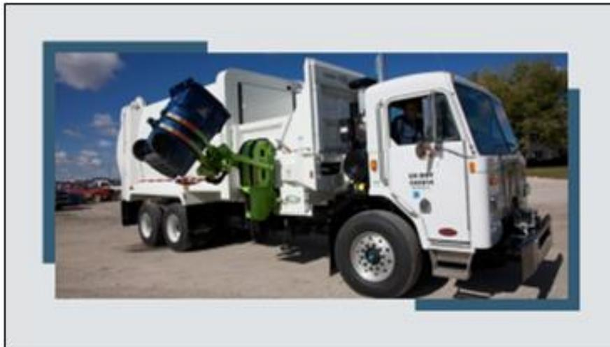
He said that this is the automated side-loading packer, which has an arm that extends out to grab the receptacle, then place it back without the driver having to step out of the vehicle. He said that these are more efficient. He said that the specifications were for New Way's Sidewinder XTR which is the dump body and on a Mack chassis LR64 truck. He said that staff received three bids. He said that Amick Equipment Company,
